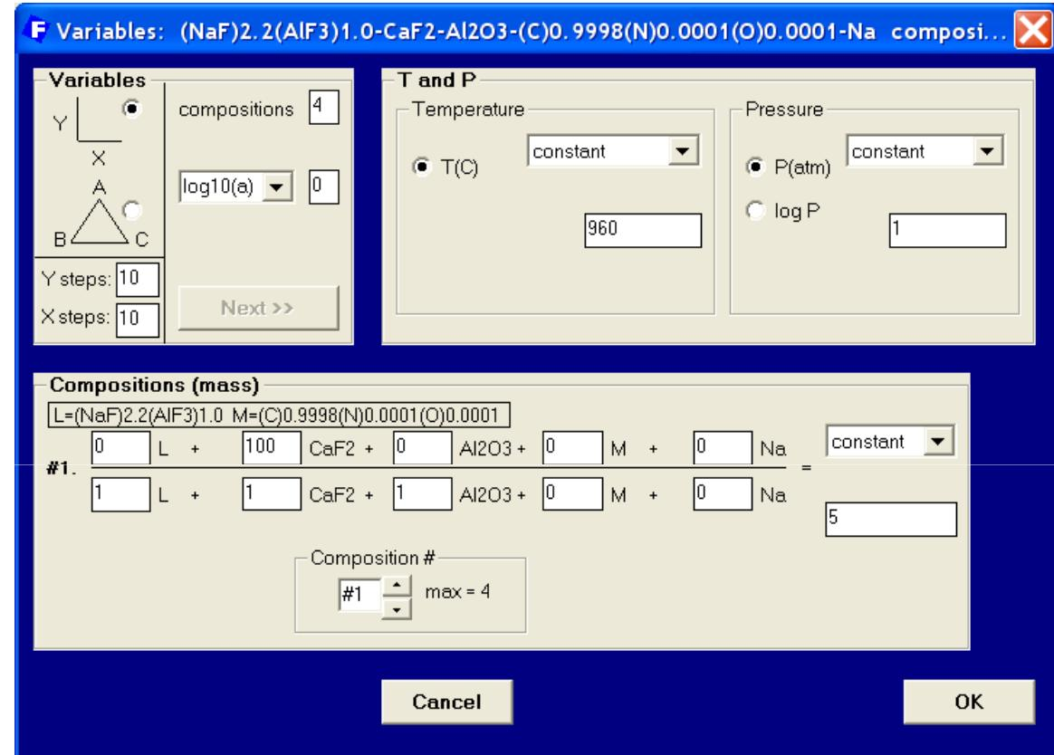
$$\frac{100 CaF_2}{1 (NaF)_{2.2}(AlF_3)_{1.0} + 1 CaF_2 + 1 Al_2O_3} = 5 \quad \text{CaF}_2 \text{ is } 5\% \text{ of the mass of the bath}$$
